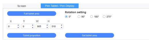
Set any part of the work area of the device to be mapped as the display area of the screen. The driver provides four modes for selection:
